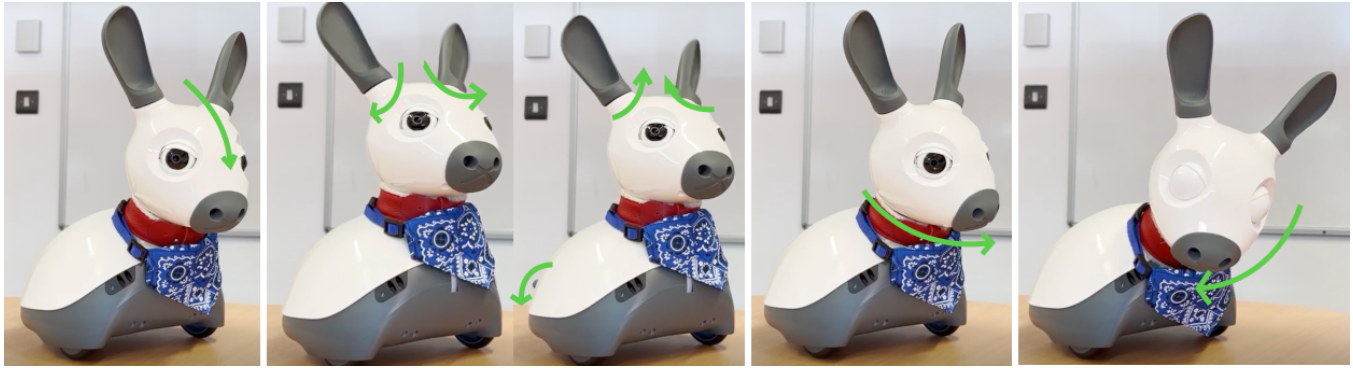
Figure 2: Examples of non-verbal backchannel behaviours defined for the study using the Miro-E robot: a) ongoing nodding (active listening), b) ears and tail wiggle, c) head tilt (curious), d) eyes closed, head down, shaking head left to right (disappointed).
