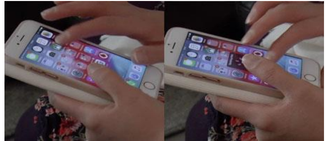
Figure 2. Performing gestures with both hands: tapping with left thumb and swiping with right index.
